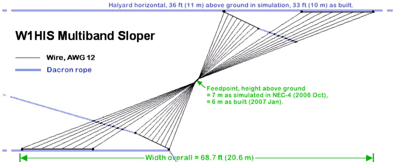
As you see, the antenna is a sloping, center-fed, doublet. It has 180° rotational symmetry about a horizontal axis through its feedpoint (perpendicular to the plane of this drawing). It would be electromagnetically balanced, except that one end (on the left in this drawing) is closer to ground. Like a single-wire, half-wavelength sloper, it radiates more strongly toward the horizon in the direction of its lower end, and less toward the horizon in the opposite direction.
